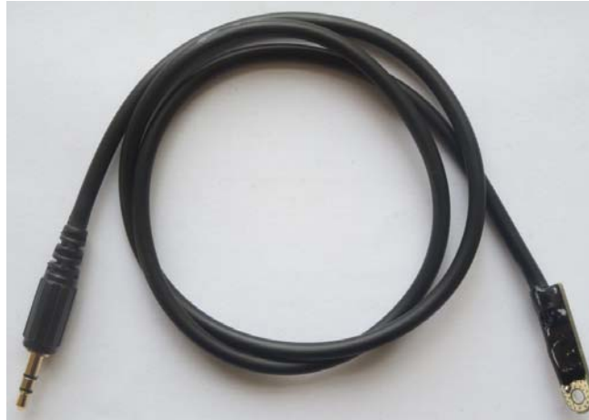
Figure 8. The Temperature Sensor
